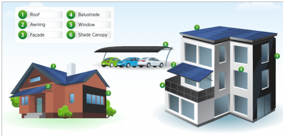
Examples of building-mounted solar arrays (Source: US Department of Energy)
